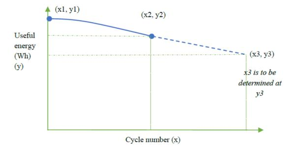
The projected cycle life (x3) is given as per below equation: x3 = x1 + ((y3-y1)\*(x2-x1)/(y2-y1))
